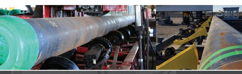
Rig preparation prepares tubulars for rig service to customer specification. It typically involves a visual thread inspection, full-length drift, and clean and re-dope with running compound.
